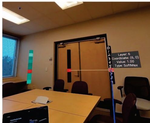
Figure 3: Frame captured from the learner's XR headset. The learner uses the virtual laser pointer (blue) to probe the firing value of neuron "6" of the SoftMax layer. The value is 1.0, indicating the correct classification of the input image (see Figure 1).
