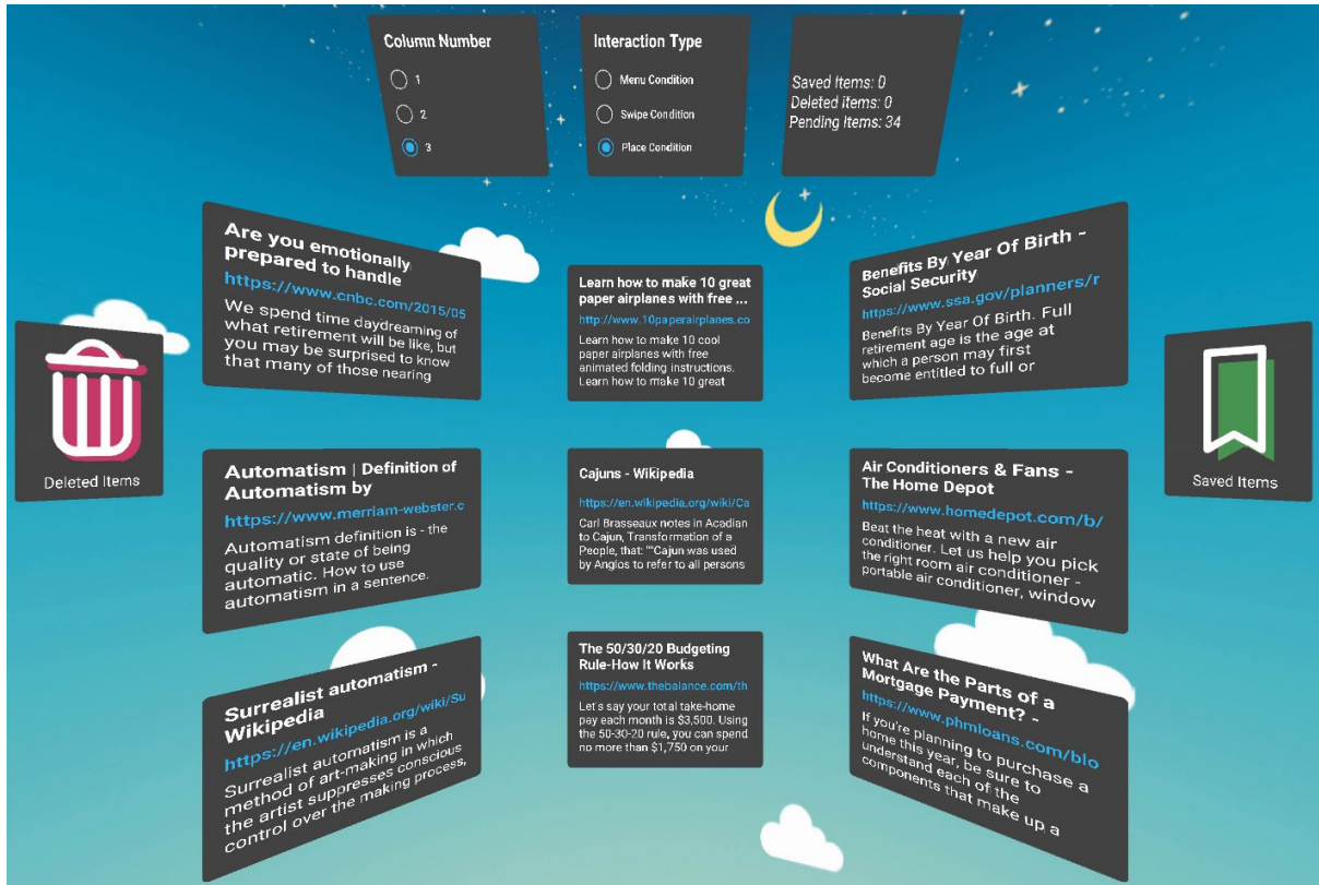
Figure 2: A zoomed-out view of the system in the 3-column layout, place interaction condition. The left and right columns wrap around the view of the user. The column number, interaction type, and statistics windows will be hidden for participants and replaced with a task description display.
